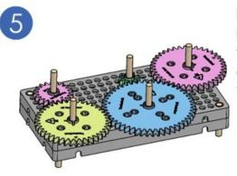
Place **gears** into the base. Position them so that the teeth **mesh**. If gears are too close, or too far away, the teeth will not mesh correctly.
